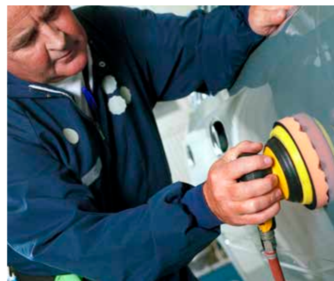
Sanders LSV 19, 28, 38 and 48 Power: 0.37 – 1.9 kW Wheel dia. 50 – 200 mm
