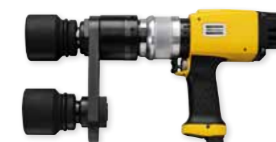
LTP 61 shut-off nutrunner with multi torque selector up to 4 different torque levels Torque range: 55 – 3,800 Nm Speed range: 50 – 1,800 rpm
