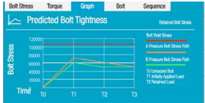
Load Graph window, displays bolt stress over a 3 stage time period
